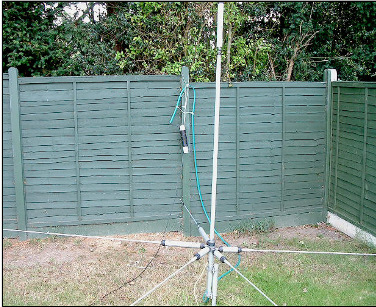
G4APL Ugly Choke Balun inline with the GB7CIP Pactor Trapped HF Ground Plane
