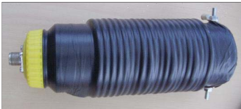
Dave uses a plastic drink bottle as a form. He installs an S0-239 in the bottle cap and antenna connectors on the other end! NICE TIP DAVE!
