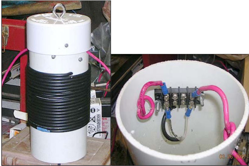
Photos courtesy Bill, KI4PCB, using 4" PVC FORM Notice the screw terminal block used for connections
